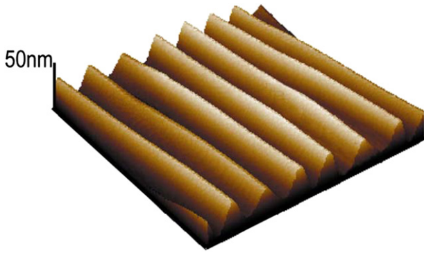
Fig. 2. AFM images of wrinkled films of 25 nm thick 990 kg/mol PS film. Scan size is 7.5 \mu\text{m} \times 7.5 \mu\text{m} and the height scale of the micrograph is 50 nm as shown.
